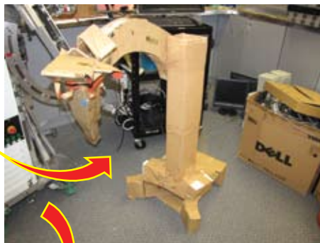
Paper prototype of the 2 nd generation robot for early testing and modification
