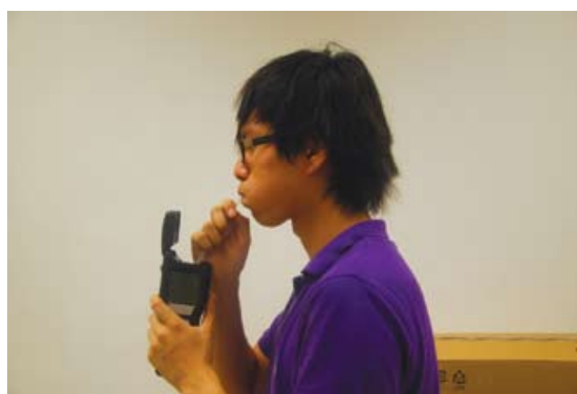
Figure 3. The integration of microsensors, piezoresistive transducer, air sampling and integrated circuit systems provide a portable and field-deployable monitoring device for breath diagnosis.
