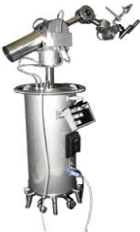
The Department of Orthopaedics & Traumatology, CUHK developed the first prototype of passive surgical robot which has been used in various orthopaedic surgical procedures with satisfactory clinical outcome. The robot improves the surgical precision and accuracy effectively by minimizing the physical tremor of the hands of surgeons.
